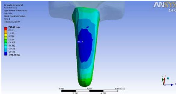
Fig. 11. Normal Compressive Stress Distribution After Application of 5N.
