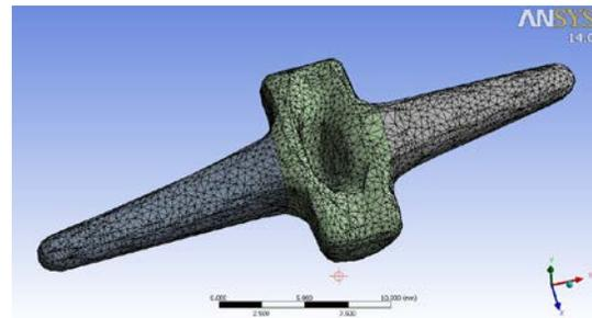
Fig. 1. ANSYS Simulation of Mesh Size 0.5 mm, close to default size.
