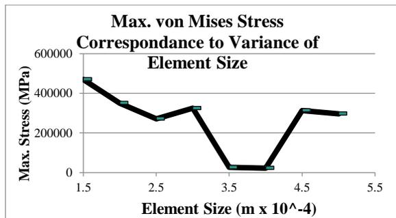
Fig. 3. Graph of Varying Element Size and its Correlation of Varying Maximum von Mises Stress.
