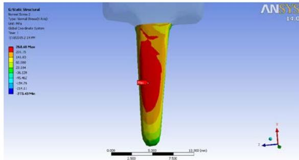
Fig. 12. Normal Tensile Stress Distribution After Application of 5N.
