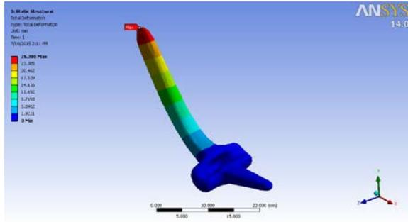
Fig. 7. Total Deformation for Mesh Size  $5 \times 10^{-4}m$ .
