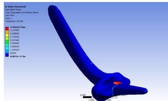
Fig. 6. von-Mises Equivalent Stress of Swanson Toe Implant of Mesh Size  $1.5 \times 10^{-4}m$ .
