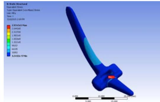
Fig. 5. von-Mises Equivalent Stress of Swanson Toe Implant of Mesh Size  $5 \times 10^{-4}m$ .
