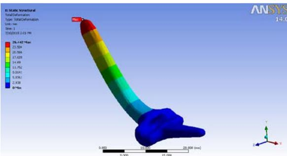
Figure 8. Total Deformation for Mesh Size  $1.5 \times 10^{-4}m$ .
