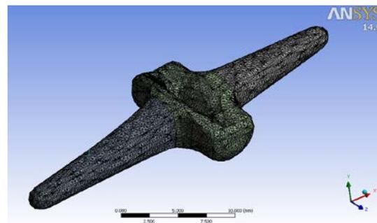
Fig. 2. ANSYS Simulation of Mesh Size 0.15 mm.
