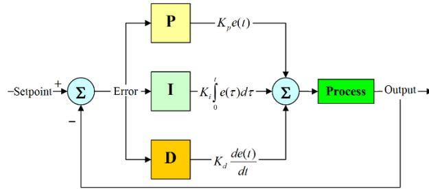
Figure 2. PID Workflow.
