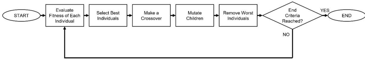
Figure 3. Block Diagram for a simple Genetic Algorithm.
