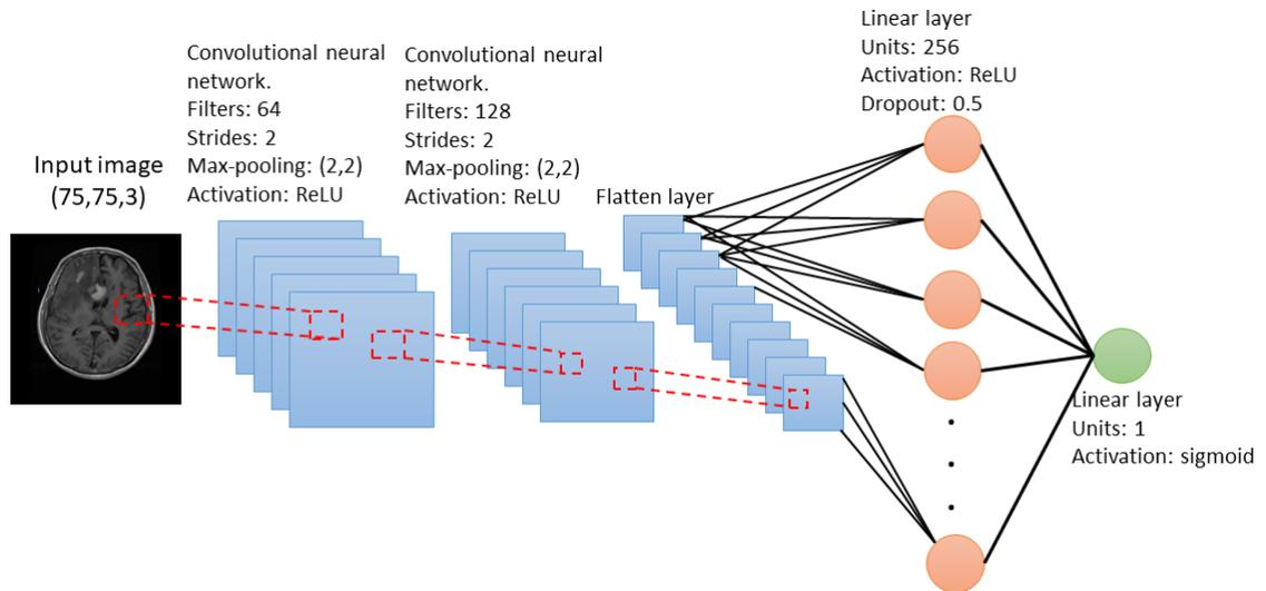
Figure 3. Neural network structure used to classify malignant tumors.
