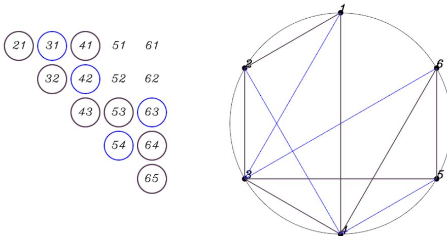
Figure 7. Intermediate stage of the drawing aids for the linkage shown in Figure 5. The secondary IVCs found in the first iteration of the program are also included.
