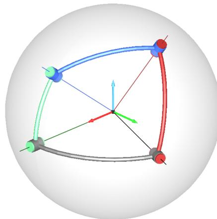
Figure 10. Drawing of a four-bar spherical linkage using the symbolic mathematics program.
