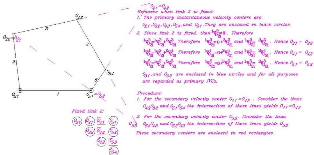
Figure 2. Determination of the secondary IVCs when  $\omega_2 = 0$ .
