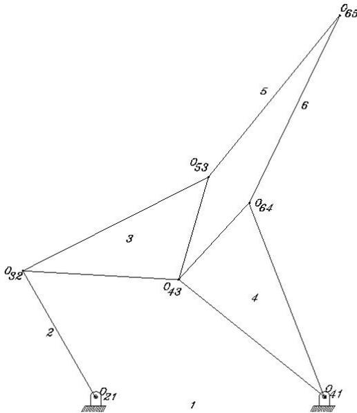
Figure 5. Planar linkage used to illustrate the process of automated determination of the IVCs.
