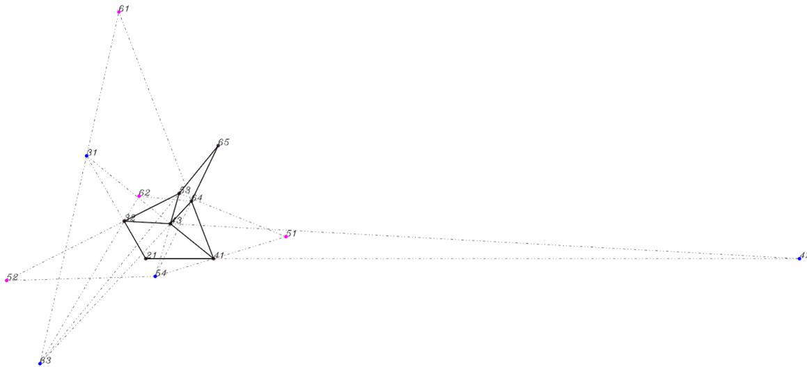
Figure 9. The results indicating the original linkage, the primary IVCs in black, the IVCs obtained in the first iteration in blue and the IVCs obtained in the second iteration in pink. The lines required to graphically obtain by intersection the secondary IVCs are also shown.
