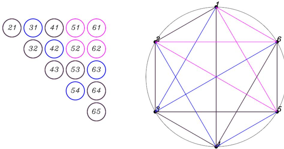
Figure 8. Final stage of the drawing aids for the linkage shown in Figure 5. The secondary IVCs found in the first and second iterations of the program are also included.
