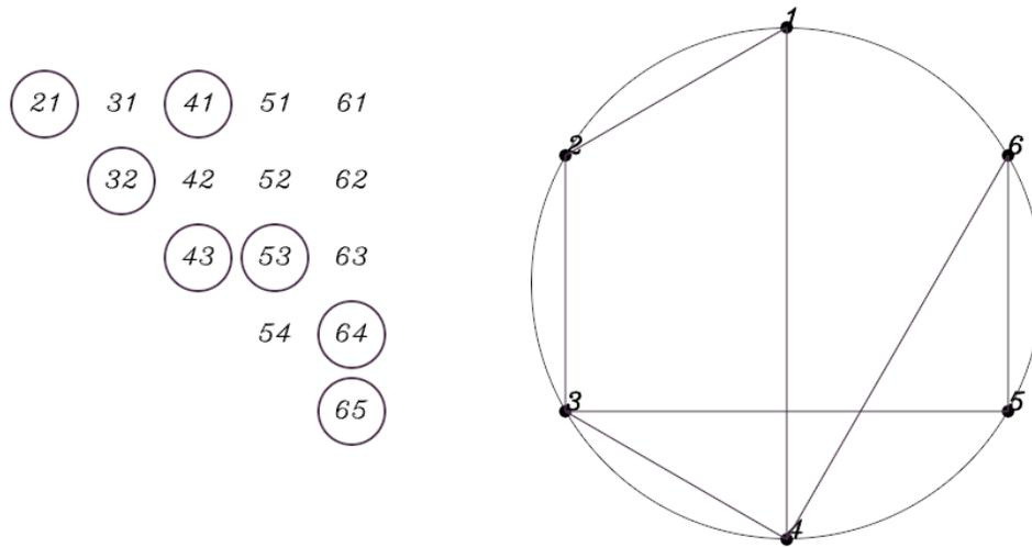
Figure 6. Initial stage of the drawing aids for the linkage shown in Figure 5. Only the primary IVCs are shown, and the corresponding secant is drawn in the circle at the right.
