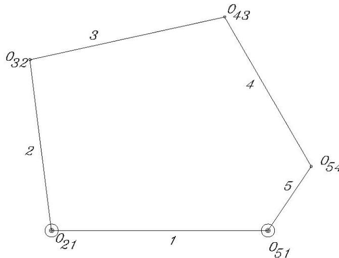
Figure 1. Planar five-bar linkage with 2 degrees of freedom.
