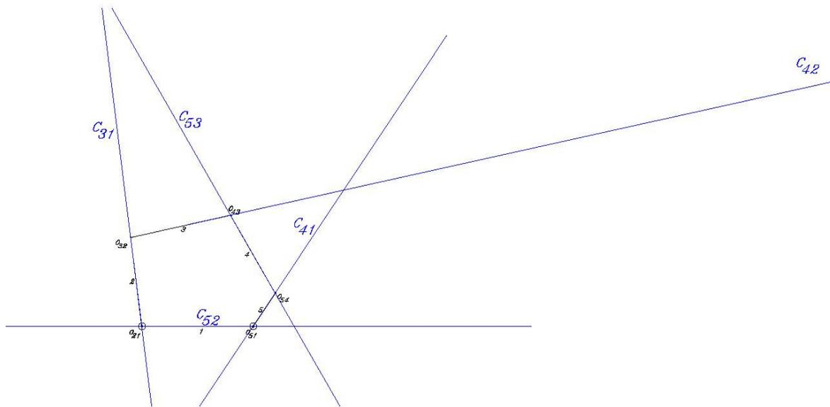
Figure 4. Determination of the center lines associated with the secondary IVCs of the five-bar linkage shown in Figure 1.
