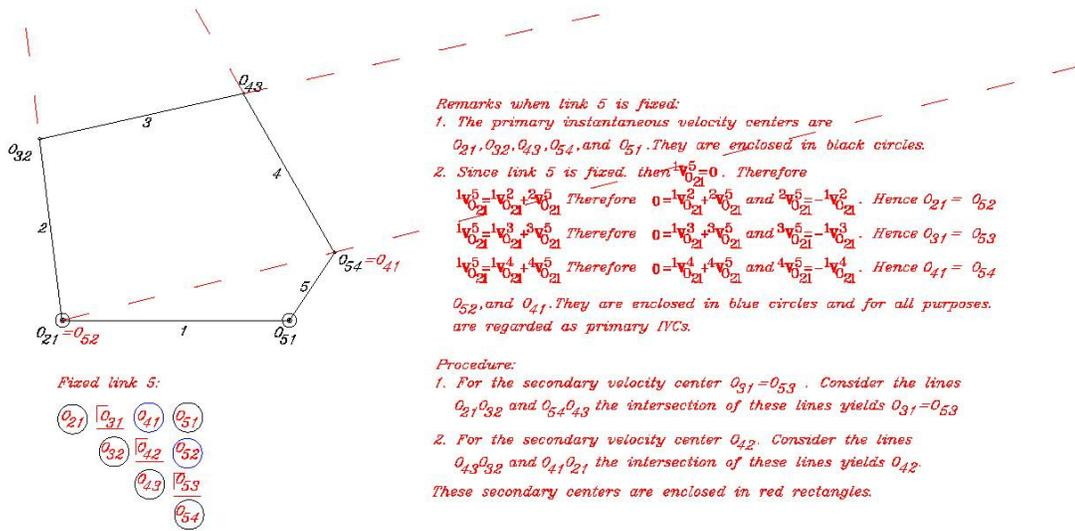
Figure 3. Determination of the secondary IVCs when  $\omega_5 = 0$ .
