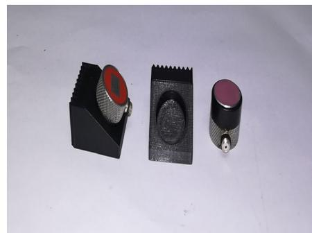
Figure 3 3D printed 30° angle wedges.
