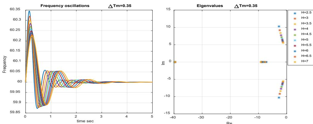
FIGURE 1: frequency oscillations to different values of  $H$  and their corresponding eigenvalues
