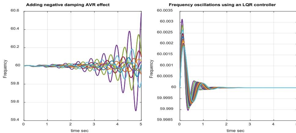
FIGURE 4: Frequency oscillations using an LQR controller in a SMIB system with AVR. Higher oscillations correspond to lower values of  $H$
