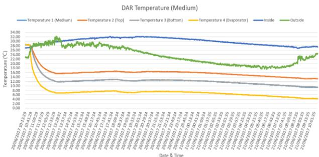
IMAGEN 7: Temperature of refrigeration systems in medium level.
