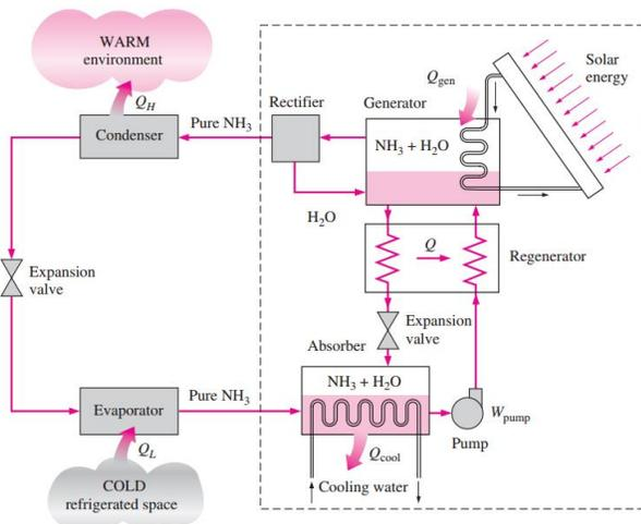
IMAGEN 2: Ammonia absorption refrigeration cycle.
