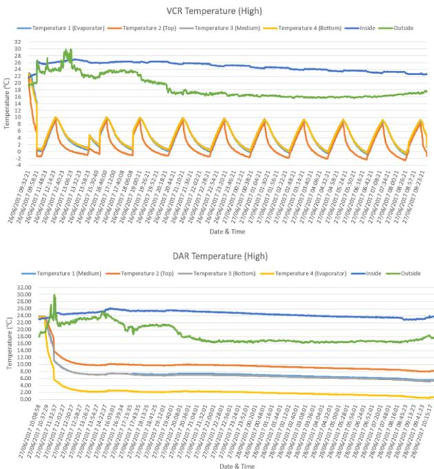
IMAGEN 10: Temperature of refrigeration systems in high level.
