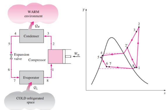
**IMAGEN 1: Vapor-compression refrigeration cycle and T-s diagram.**
