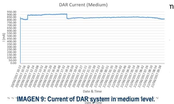
IMAGEN 9: Current of DAR system in medium level.
